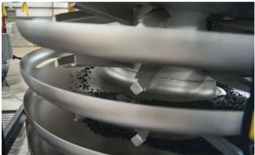
High throughput requires carefully planned conveying and heat management. On this line, a spiral elevator cools and dries newly formed pellets before they are boxed, preventing clumping.
